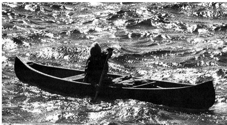
Kneeling in the Center with load forward gives better control in any wind (B. Mason)
