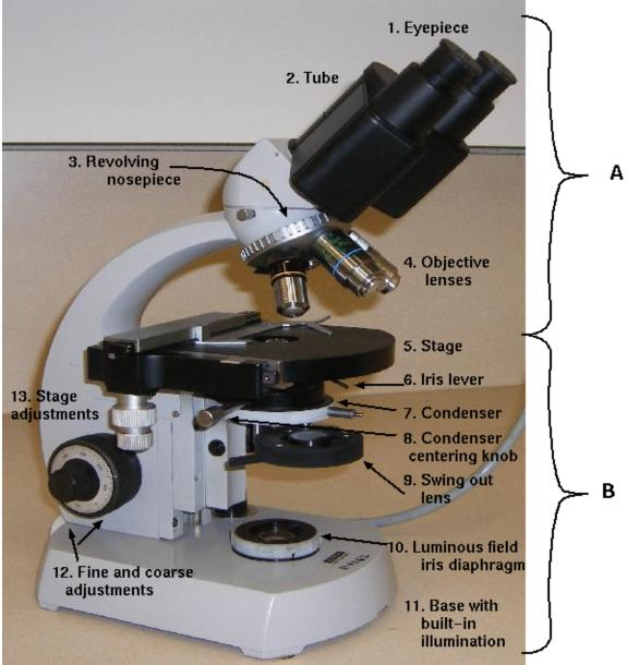
5. (10 points) The components of the microscope could be said to be organized into two sections, labeled A and B on the figure. For section, describe in one sentence the common purpose to which all components in that section contribute.
