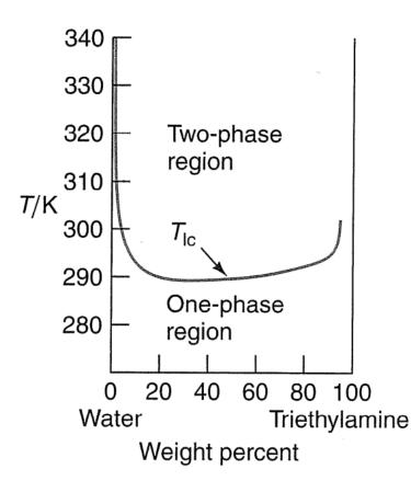
**4. (a)** From the phase diagram to the left (water-triethylamine), determine the ratio of the masses of the phases present at 295K, for a mixture containing 30.0 wt % triethylamine. (b) What are the respective compositions of the phases? (*Figure copied from Laidler, Meiser, Sanctuary, Physical Chemistry, 4<sup>th</sup> edition.*)
