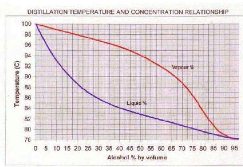
Starting with a 5.0% ethanol by volume solution (a typical value for beer or cider), what is the minimum number of steps
