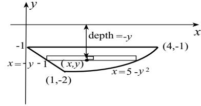
$$\begin{aligned} F &= \int_{-2}^{-1} \int_{-y-1}^{5-y^2} \rho g(-y) dx dy = -\rho g \int_{-2}^{-1} \{xy\}_{-y-1}^{5-y^2} dy \\ &= -\rho g \int_{-2}^{-1} y[(5 - y^2) - (-y - 1)] dy = -\rho g \int_{-2}^{-1} (-y^3 + y^2 + 6y) dy \\ &= -\rho g \left\{ -\frac{y^4}{4} + \frac{y^3}{3} + 3y^2 \right\}_{-2}^{-1} = \frac{35\rho g}{12}. \end{aligned}$$
