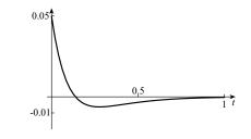
The auxiliary equation is  $2m^2 + 4m + 200 = 0$  with solutions  $m = -1 \pm 3\sqrt{11}i$ . A general solution of the differential equation is  $x(t) = e^{-t}[C_1 \cos(3\sqrt{11}t) + C_2 \sin 3\sqrt{11}t)]$ . To satisfy the initial conditions, we must have
