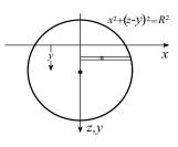
where V is the volume of water displaced by the sphere when its centre is y m below the surface. We can calculate V with the following double iterated integral,
