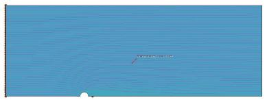
11. Now, create a second streamline that uses the line the recirculation zone. Use Steps 5 to 8 above except put the seed part as the "recirculation zone line y direction". Also change the "Direction" to "Both". After Clicking Create and Close, rename "Streamline" to "Streamlines in recirculation zone". You should get something that looks like:
