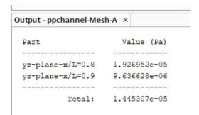
The Total quantity can be ignored. The objective this would normally be just to get the area-average pressure values to use for a dP/dx calculation.
