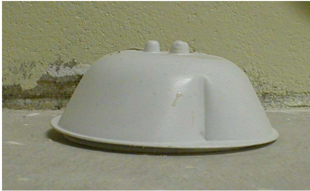
Figure 1. Trap baited with pheromones for the confused and red flour beetles ( Tribolium confusum and Tribolium castaneum ), common pests of pasta plants, flour mills.
