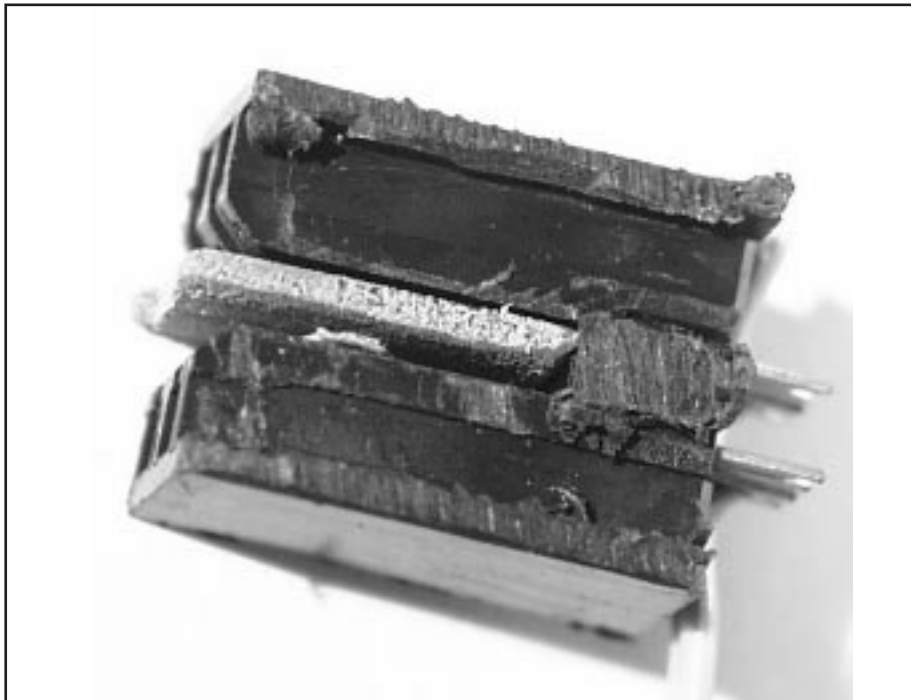
Figure 12. Picture of a piece of floppy drive connector with a copper bridge completing the circuit used in Expt #43
