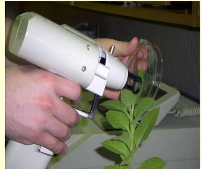
The real trick is to fire pellets with enough force to break into cell, but not so much as to go right through tissue. Must optimize distance, placement of tissue, dispersal of charge (don't want charge to all go in one place).
