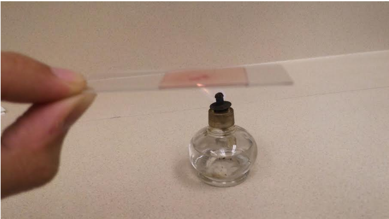
Figure 8: Pass the microscope slide 8-10 times over an alcohol lamp. DO NOT hold the slide over the flame too long or the stain will boil off.
