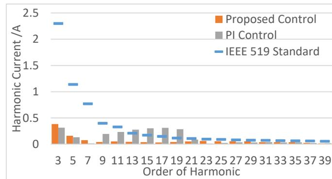
Fig. 16 Input current harmonic comparison between the proposed control scheme and the PI control scheme at 1.5kW
