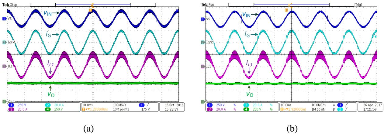
Fig. 14 Experimental waveforms of (a) the proposed control scheme and (b) the PI control scheme at 1.5kW output.
