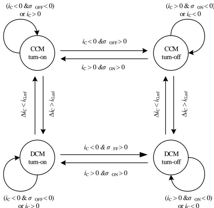
Fig. 7 The logic flow of the mode operation.
