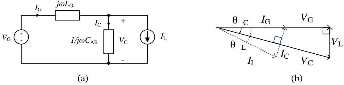
Fig. 4 AVG-BPFC's (a) phasor domain equivalent circuit and (b) the corresponding vector diagram.
