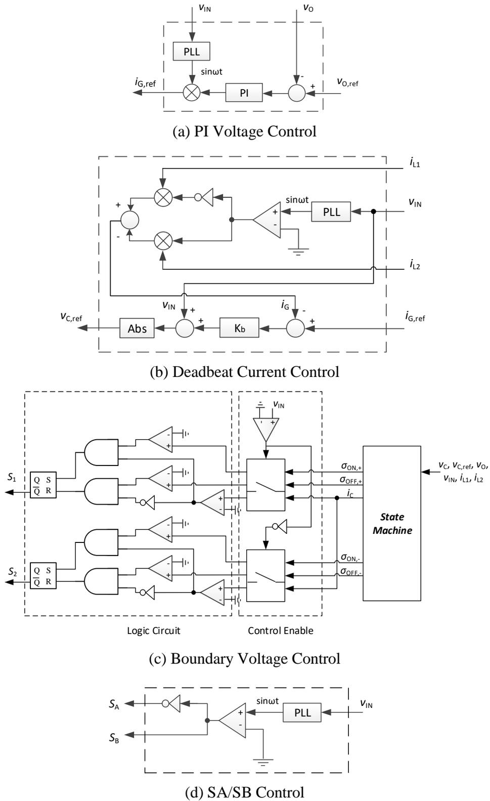
Fig. 5 Flow Chart of the control diagram.
