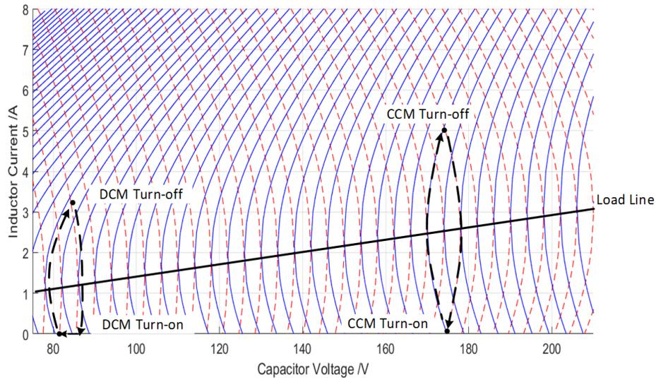
Fig. 6 The switching surface of the boundary control.
