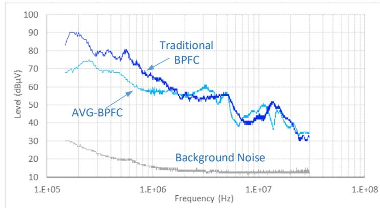
Fig. 13 Conductive EMI measurement of the traditional BPFC and AVG-BPFC at 1kW output.
