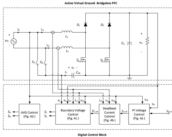
Fig. 1 The proposed control scheme in AVG-BPFC.
