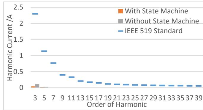
Fig. 17 Input current harmonic comparison between the proposal control scheme with and without state machine at 230W.
