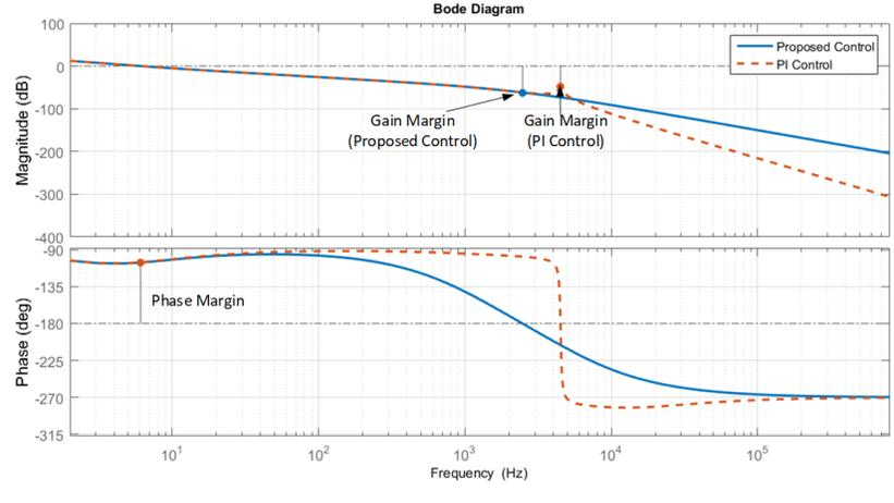
Fig. 9 Frequency plot of (a) the boundary block, (b) the current closed loop transfer function and (c) the overall open loop system transfer function.
