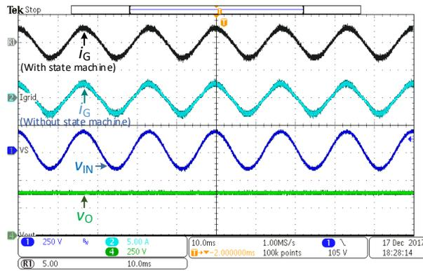
Fig. 15 Experimental waveforms of the proposed control scheme at 230W with and without state machine.
