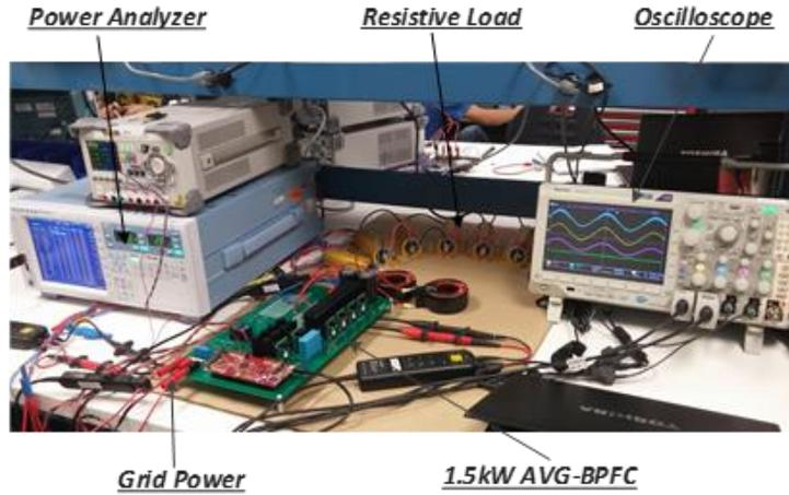
Fig. 11 Experimental test setup.
