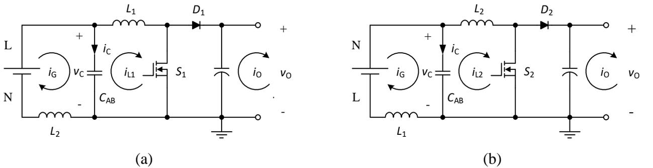
Fig. 2 Equivalent circuit of AVG-BPFC in (a) positive line cycle and (b) negative line cycle.
