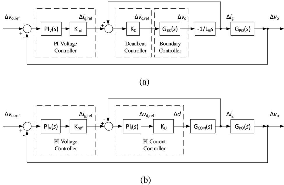
Fig. 8 Block diagram of (a) the proposed control scheme and (b) PI control scheme
