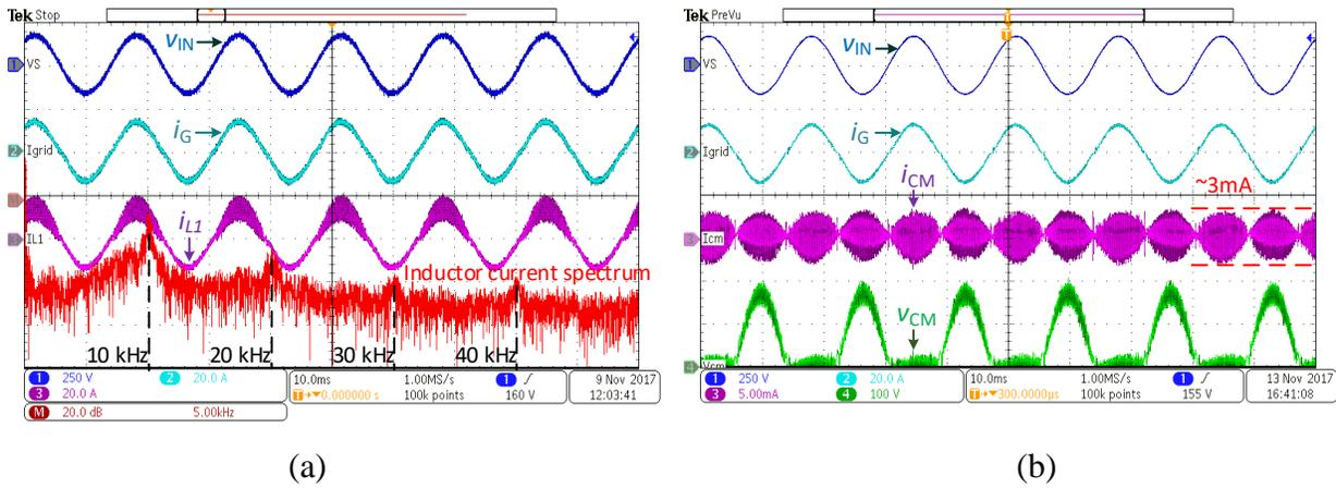
Fig. 12 Experimental waveforms of the proposed control scheme with (a) the inductor current's FFT analysis and (b) the leakage current measurement at 1kW output.
