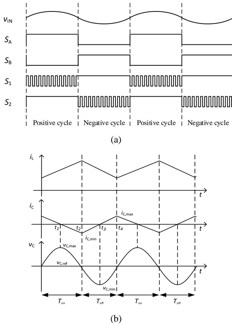
Fig. 3 Key waveforms of AVG-BPFC's (a) switches operational sequence and (b) capacitor switching behaviours.
