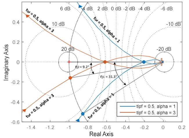
Fig. 10 Nyquist diagram of system open-loop transfer function with delay effect with different  $\alpha$  when LPF in slave module is functioning.
