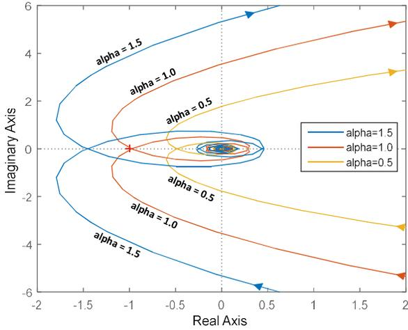
Fig. 7 Nyquist diagram of system open-loop transfer function with communication effect with different  $\alpha$ .
