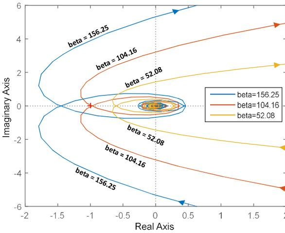
Fig. 8 Nyquist diagram of system open-loop transfer function with communication effect with different  $\beta$ .
