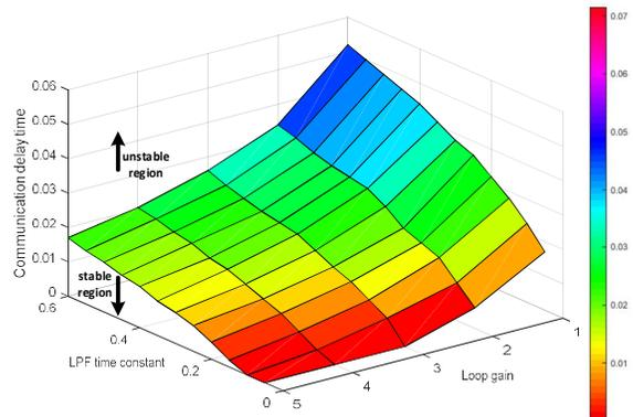
Fig. 11 Bound for the system operating in stable region,  $\beta$  is fixed to 156.25,  $\Delta t_2$  is fixed to 0.034s.
