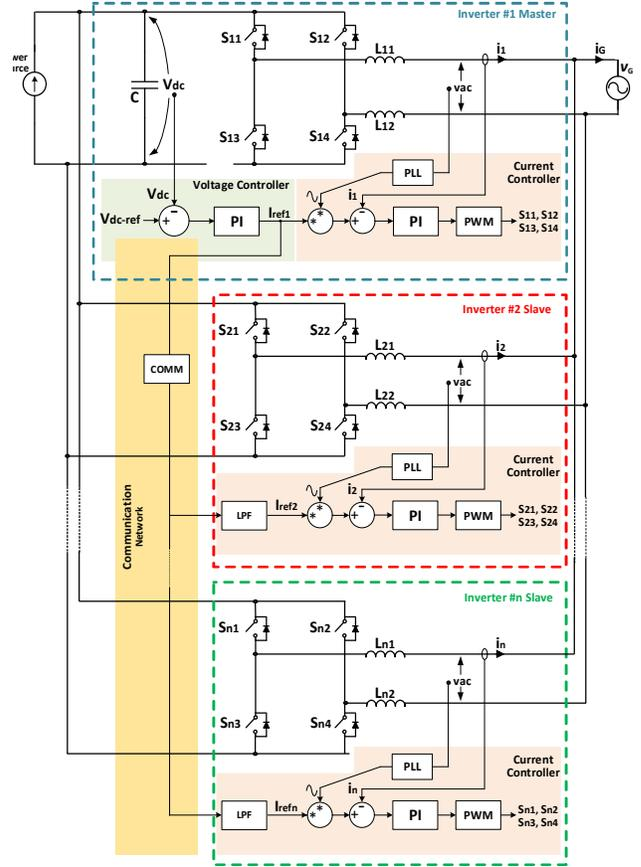
Fig. 4 Overview of a typical input-parallel output-parallel inverter system with master-slave control architecture.
