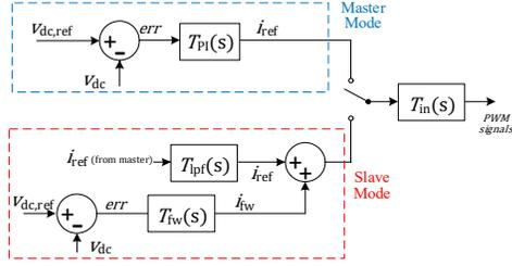
Fig. 14 Controller diagram with multi-master control ability.
