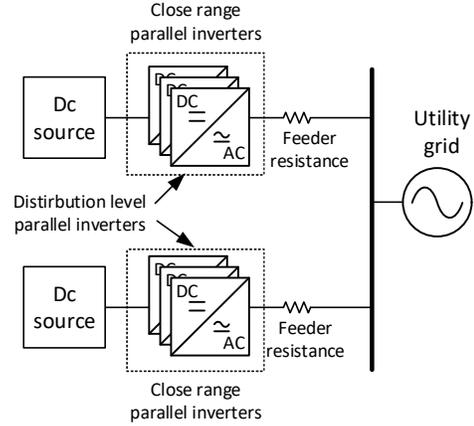
Fig. 1 Application of close-range parallel inverter system.
