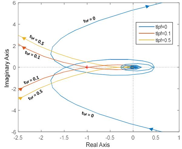
Fig. 9 Nyquist diagram of system open-loop transfer function with communication effect with different  $t_{lpf}$  in slave module.
