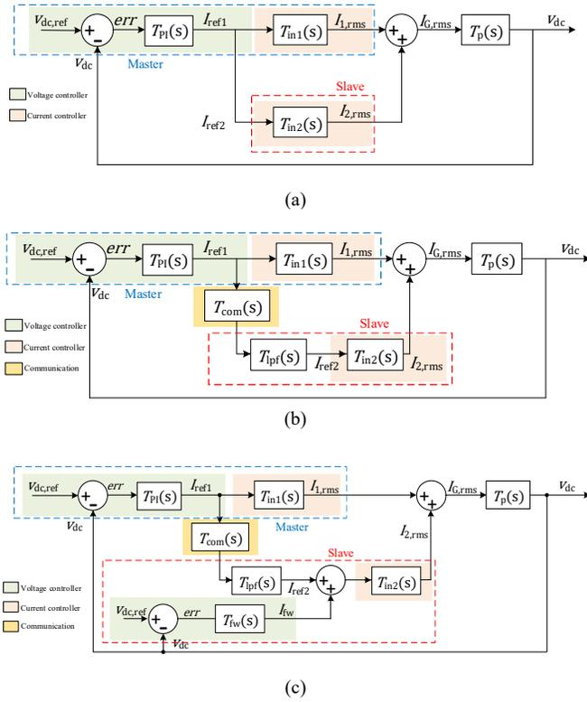
Fig. 5 Control diagram of one master module and one slave module operating in parallel, (a) without communication impact, (b) with communication impact, (c) with voltage feed-forward loop in slave module.
