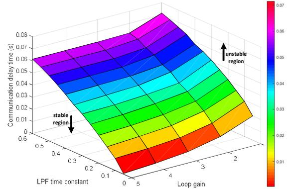
Fig. 13 Bound for the system stable region while FFL is involved,  $\beta$  is fixed to 156.25,  $\Delta t_2$  is fixed to 0.034s and  $K$  is fixed to 0.0005.
