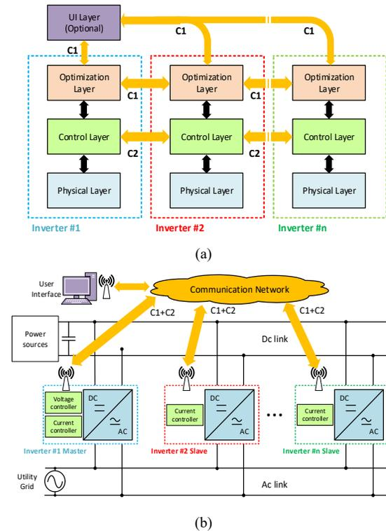
Fig. 2 (a) Typical logical structure of parallel inverter system with two separate communication networks C1 and C2. (b) Proposed master-slave controlled parallel inverter system with one LBCom network.
