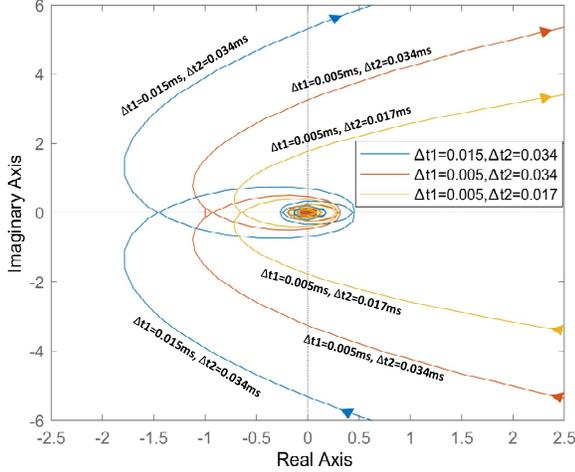
Fig. 6 Nyquist diagrams of system open-loop transfer function with communication effect and no LPF.
