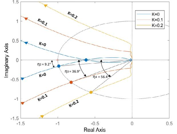
Fig. 12 Nyquist diagram of system open-loop transfer function with both LPF and FFL in slave module, while  $t_{\text{lpf}} = 0.5\text{s}$  and  $\alpha = 3$ .
