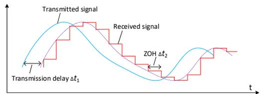
Fig. 3 Delays of low-bandwidth digital communication.
