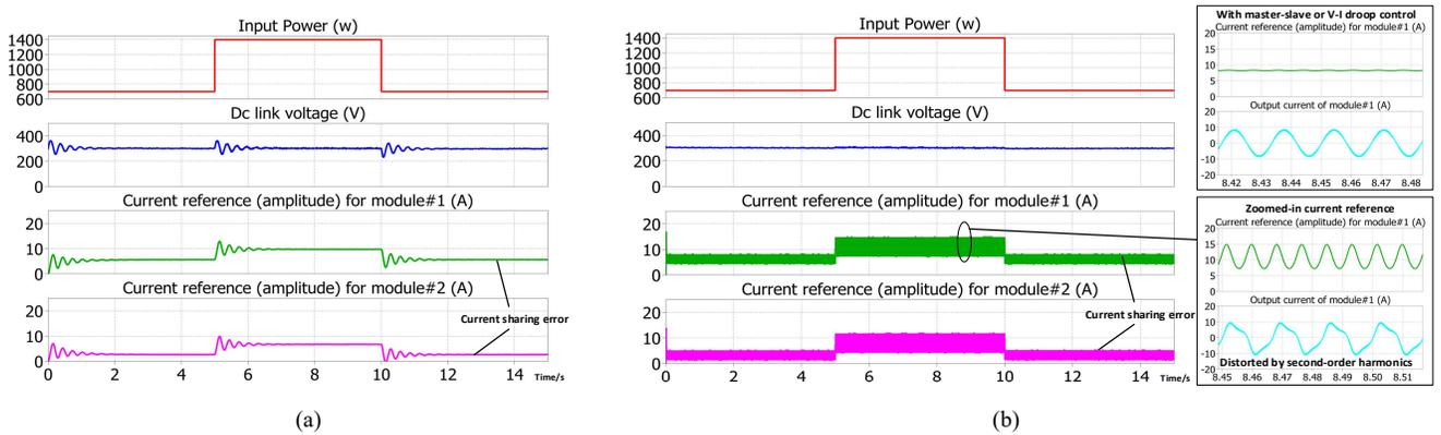
Fig. 16 Simulation results of two inverters operating in parallel using droop control with secondary voltage regulation, both droop coefficients are set to 10 Ohm, and 1% voltage sensing error is considered, (a) V-I droop control, (b) I-V droop control.
