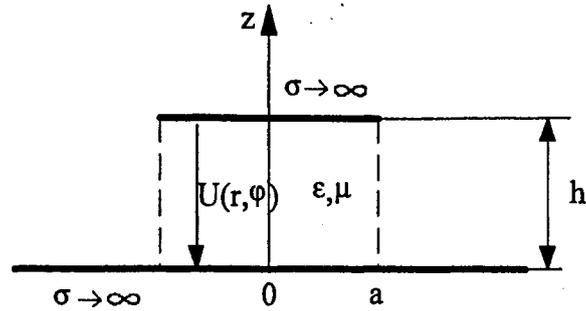
Fig. 1. Circular microstrip resonator.
