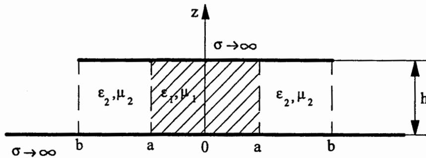
Fig. 2. Circular resonator with inhomogeneous dielectric.
