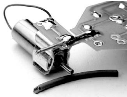
Close-up of stripped copper wire soldered onto motor mount support pads
