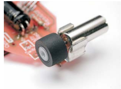
...then add the wheel. A drop of glue in the wheel hole to secure the works, and you're done!
