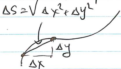
$$\left\{ \begin{array}{l} \text{In 2D, } \\ ds = \sqrt{dx^2 + dy^2} \end{array} \right. \quad \left\{ \begin{array}{l} \text{In 3D, } \\ ds = \sqrt{dx^2 + dy^2 + dz^2} \end{array} \right.$$
