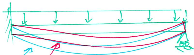
~~Deformed shape if the rotational constraint at location A, equal reaction forces at locations A and B ,  $R_A = R_B = \frac{w_0 L}{2}$~~
