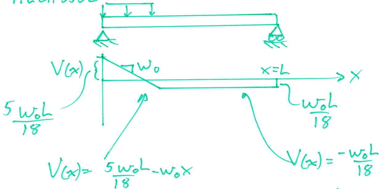
We have 2 separate equations for the shear; one between 0 and  $\frac{L}{3}$  and another between  $\frac{L}{3}$  and L. We are also going to have 2 equations for the moment.
