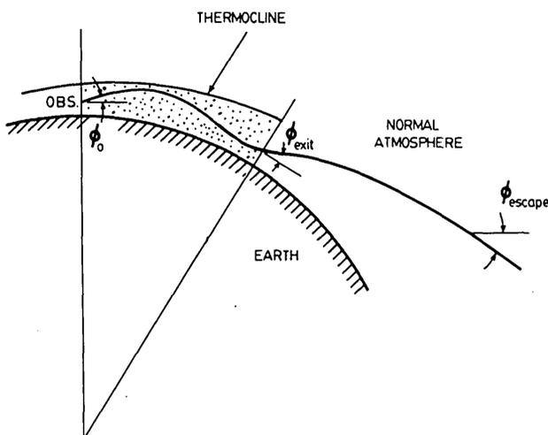
Fig. 1. Geometry of the Novaya Zemlya model. A light ray, with direction of propagation reversed for computational convenience, emanates from the observer's eye with elevation angle  $\phi_0$ . After exiting from the duct, the ray undergoes the normal atmospheric refraction before escaping into space.
