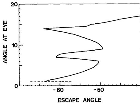
Fig. 3. Phase I transfer characteristic. The angles are in min of arc relative to the observer's coordinate system. The observer sees the duct extending from 1 to 14 min of arc in elevation.
