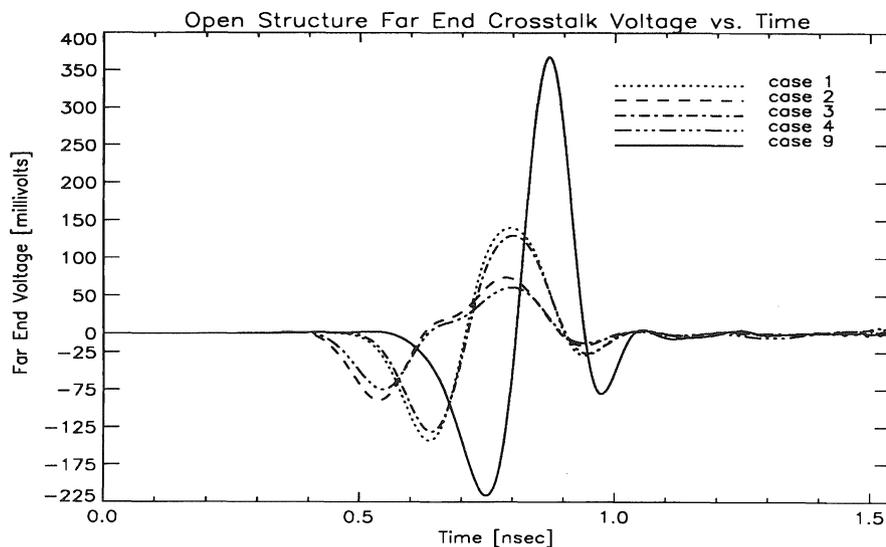
Figure 7. Open structure far end crosstalk, cases 1, 2, 3, 4, and 9.
