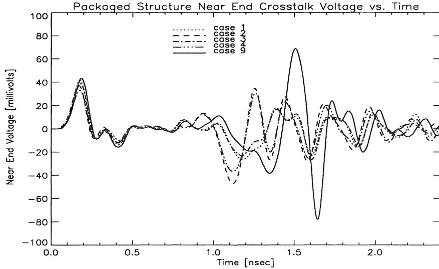
Figure 5. Packaged structured near end crosstalk, cases 1, 2, 3, 4, and 9.
