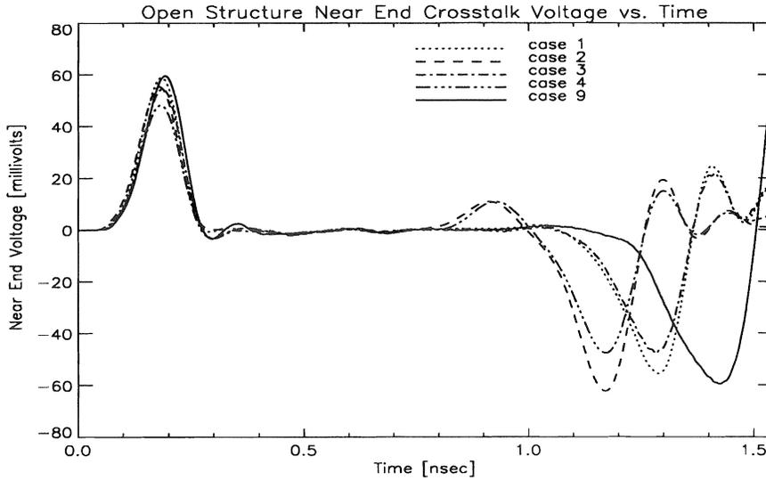
Figure 3. Open structure near end crosstalk, cases 1, 2, 3, 4, and 9.
