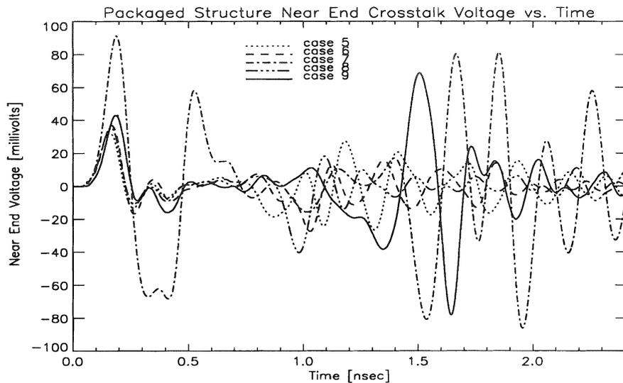
Figure 6. Packaged structure near end crosstalk, cases 5, 6, 7, 8, and 9.
