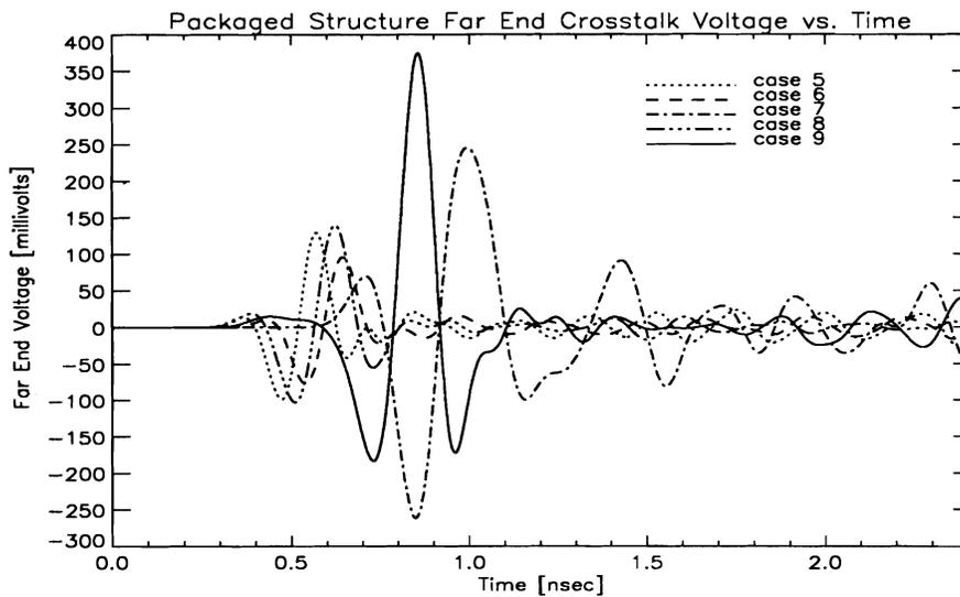
Figure 10. Packaged structure far end crosstalk, cases 5, 6, 7, 8, and 9.
