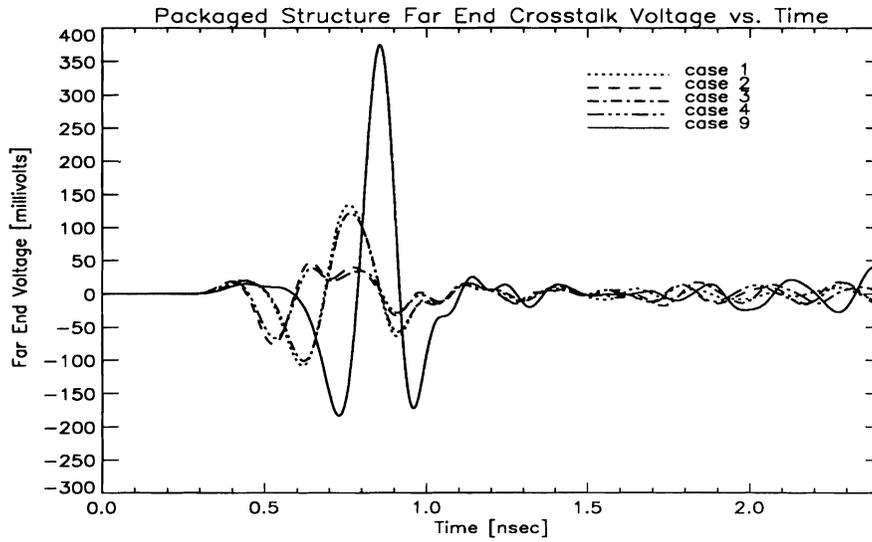
Figure 9. Packaged structure far end crosstalk, cases 1, 2, 3, 4, and 9.
