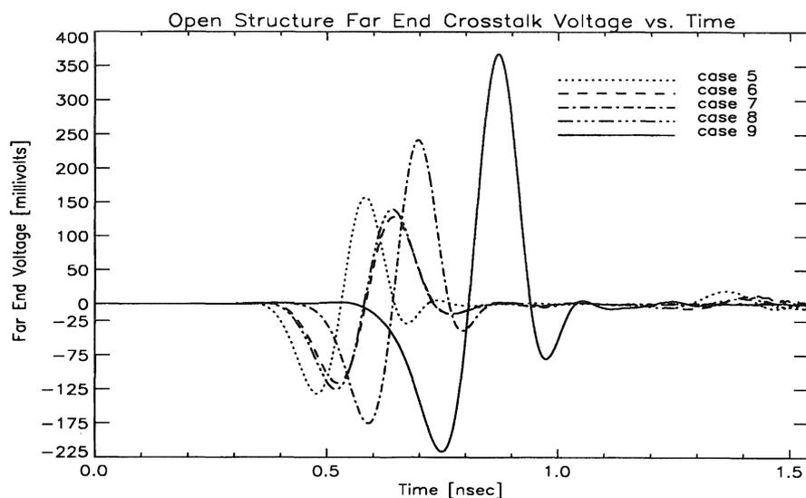
Figure 8. Open structure far end crosstalk, cases 5, 6, 7, 8, and 9.
