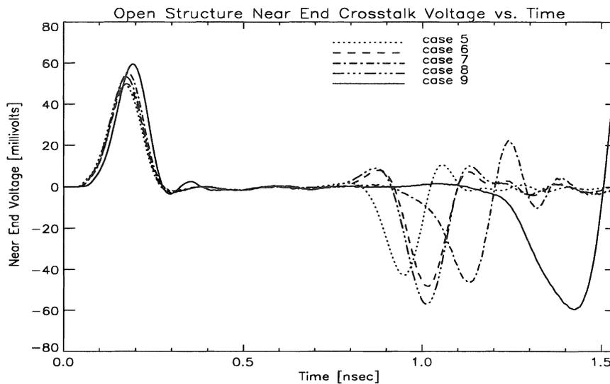
Figure 4. Open structure near end crosstalk, cases 5, 6, 7, 8, and 9.
