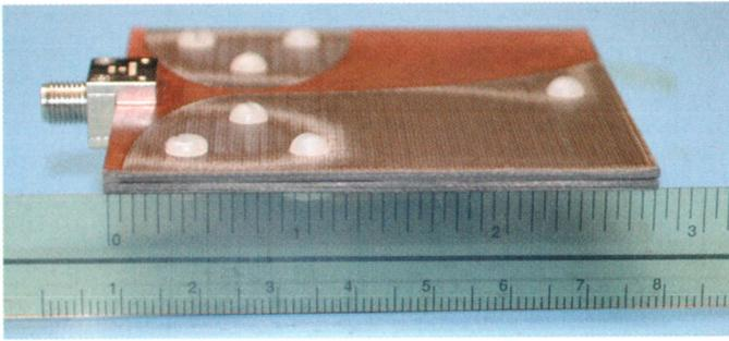
**Figure 2.** A close-up of one of the double-layered Vivaldi antennas used in the microwave imaging system. The two layers were held together with nylon screws.
