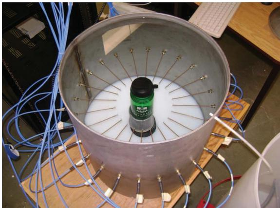
FIG. 4. Photograph of apparatus with a glycerol/water-based phantom.
