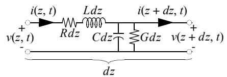
where  $Z = R + j\omega L$ ,  $Y = G + j\omega C$ ,  $R$ ,  $L$ ,  $G$ ,  $C$ , are the per-unit-length resistance [ $\Omega/m$ ], inductance [ $H/m$ ], conductance [ $S/m$ ], and capacitance [ $F/m$ ] respectively, and  $\omega$  is the angular frequency [rad/sec]. (Use the lumped-element model shown.)
