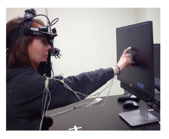
Eye position was recorded using an Eyelink II and grasp movements were recorded using an Optotrak Certus. This data was integrated into a common reference frame via Motion Monitor software (Innovative Sports Training).
