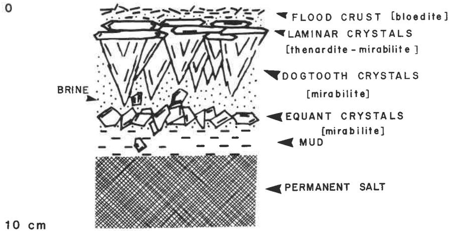
FIG. 18. Schematic profile of typical salt crust stratigraphy.
