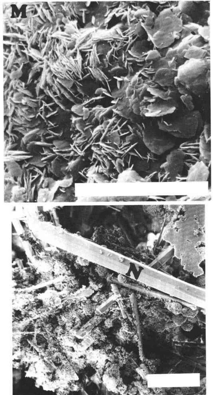
FIG. 8. Examples of mixed-layer clays (M) and nesquehonite (N) from Freeflight Lake. Scale bars = 5  $\mu\text{m}$ .
