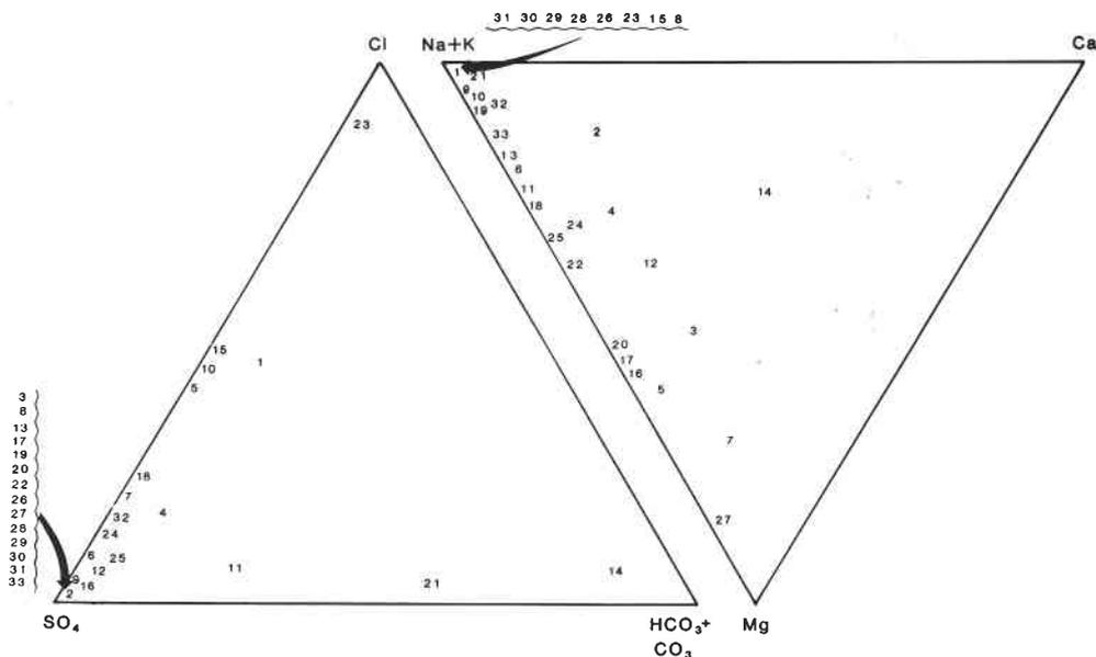
FIG. 4. Triangular diagram showing the average water composition (mol%) of selected playa lakes. Numbers refer to the lakes listed in Table 1. In the anion field lakes 3, 8, 13, 17, 19, 20, 22, 26, 27, 28, 29, 30, 31, and 33 all plot at the same point as lake 2. In the cation field lakes 8, 15, 23, 26, 28, 29, 30, and 31 all plot at the same point as lake 1. Compiled, in part, from Cole (1926), Tomkins (1953, 1954), Hammer (1978), and Last and Schweyen (1983).
