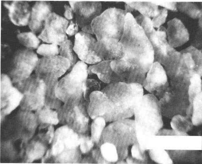
FIG. 14. Abraded gypsum crystals collected from the shoreline of Patience Lake. Scale bar = 1 mm.
