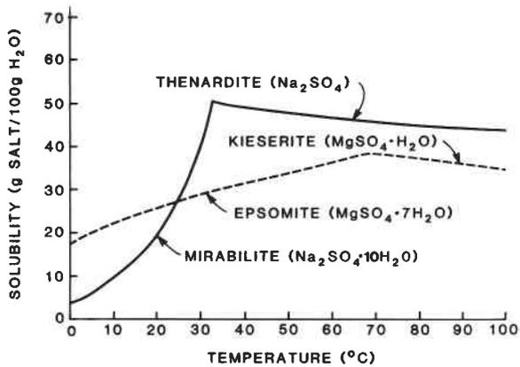
FIG. 5. Temperature-solubility curves for sodium sulfates and magnesium sulfates in pure water (after Cooke 1981).
