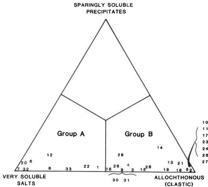
FIG. 7. Triangular diagram showing modern sediment type of selected playas. Numbers refer to lakes listed in Table 1. Lakes 10, 11, 17, 23, 24, 25, and 27 all plot at the same point as lake 2.
