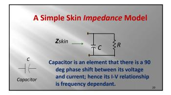
Impedance of a Capacitor:  $Z_c = \frac{1}{jc\omega}$
