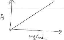
If the cell length is I em, the coefficient obtained was 0.04 = the cell has 1/2 the length, = 0.5 cm
