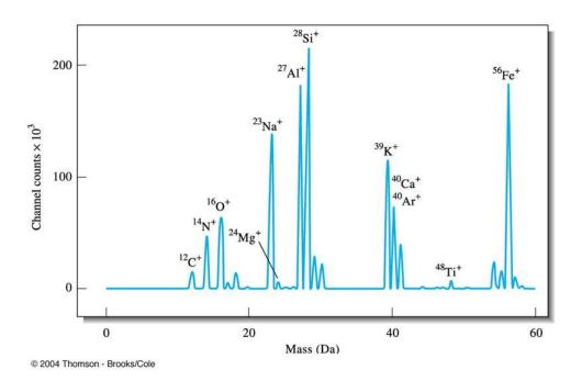
The mass spectrum of a standard rock sample obtained by laser ablation / ICP-MS.
