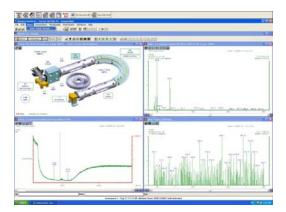
The top left screen indicates the triple quadropole MS status and the top right indicating the current data on analysis. In the bottom left window signals and data from a last run are shown, in the bottom right is live data of the MS.
