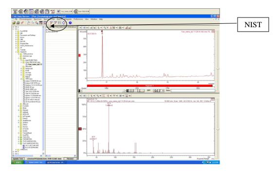
The software gives you the possibility of focusing on a section of the chromatogram (drag and drop the cursor for the area of interest) and also by clicking on the apex of a peak to obtain its mass spectrum (bottom). A **NIST** search (see bottom on second row from the top) will allow you to identify the substance corresponding to this peak with a high level of certainty.
