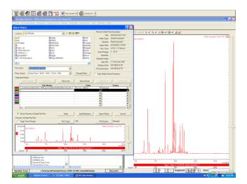
You can add up to 7 overlays by going to each slot selecting the file you want to analyze and clicking **add/replace**. When you have all the files you want to analyze click on the button that says **Open file(s)** and all the files of interest should open up.
