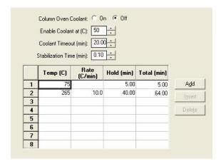
Change the program so that the oven is thus programmed to start at 75°C and stay at that temperature for 5 minutes, and then the temperature will increase by 20 °C/min until it reaches 265°C, at which it will stay for 2 min. This should give a total run time of 16.5 min.
