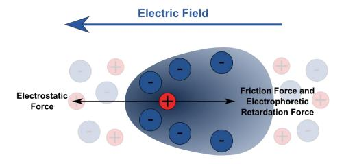
The ions reach a steady state velocity where the electric force equals the frictional force.
