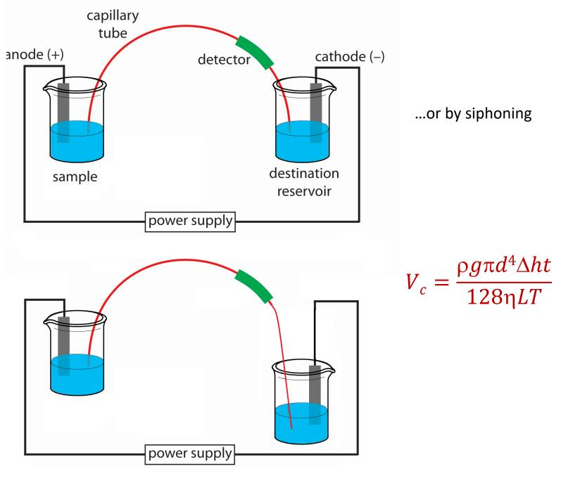
*Electrokinetic injection* is performed by simply turning on the voltage for a certain period of time.
