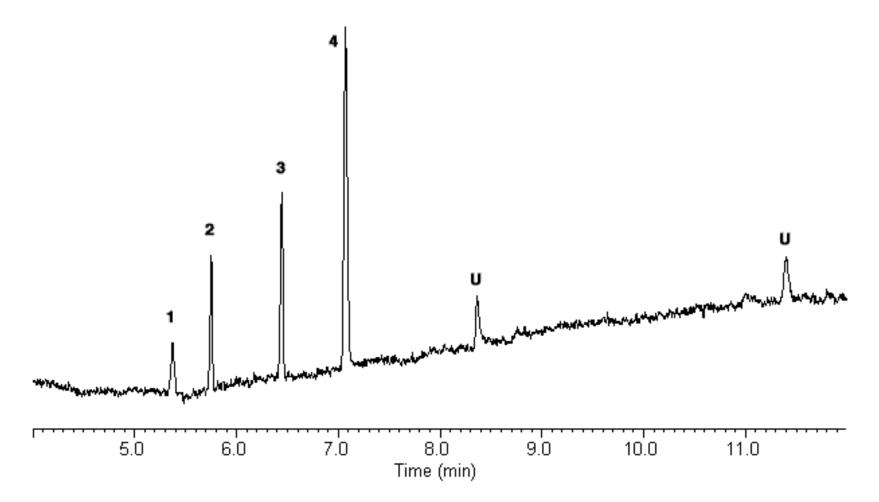
Capillary electrophoresis analysis of black tea with sugar (diluted 20×) and spiked with less than 10 ppm of sodium azide (trace at 250 nm; *y*-scale in mV). Peak assignments: (1) Cl<sup>-</sup>, (2)  $SO_4^{-2}$ , (3)  $C_2O_4^{-2}$ , (4)  $N_3^{-}$ , and (U) Unknown.
