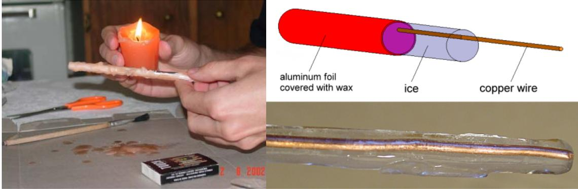
**Fig. 5.1(a)** Preparing Copper Wire.
