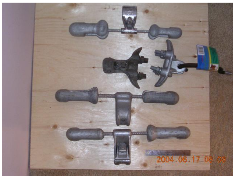
Figure 3.5: Sample obstacles (2 line clamps and 3 vibration dampers)
