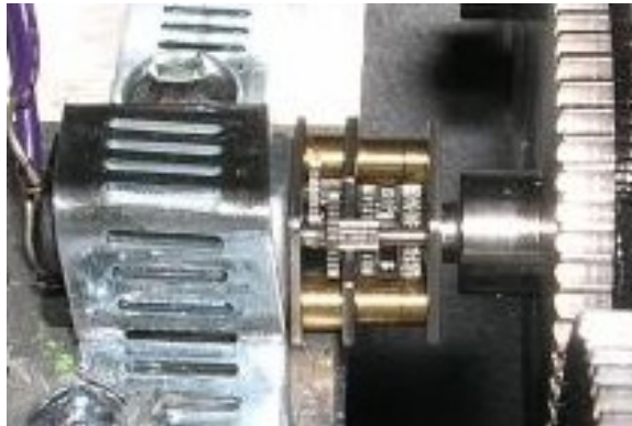
Figure 3.31: Second generation, Sanyo locomotion drive installed
