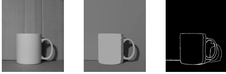
1.1: Original image 1.2: Segmentation using nonlinear diffusion 1.3: Binary contour using nonlinear diffusion
