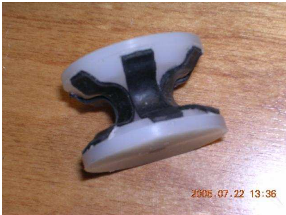
Figure 5: Added traction to line grip wheels
