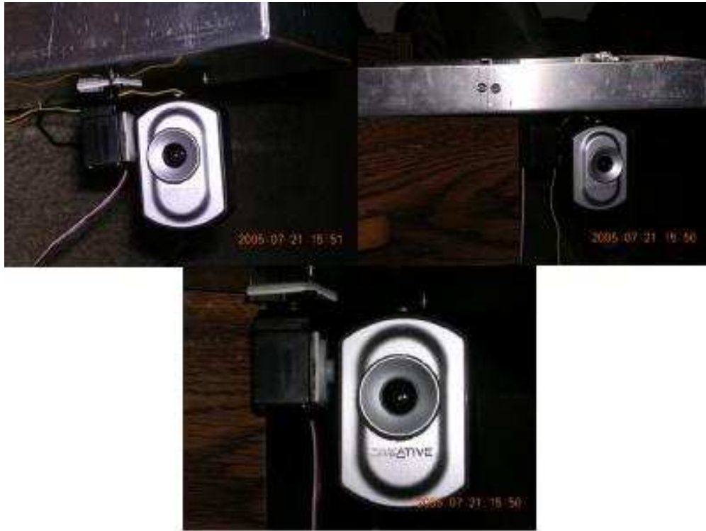
Figure 7: Camera mounted underneath Alice II platform
