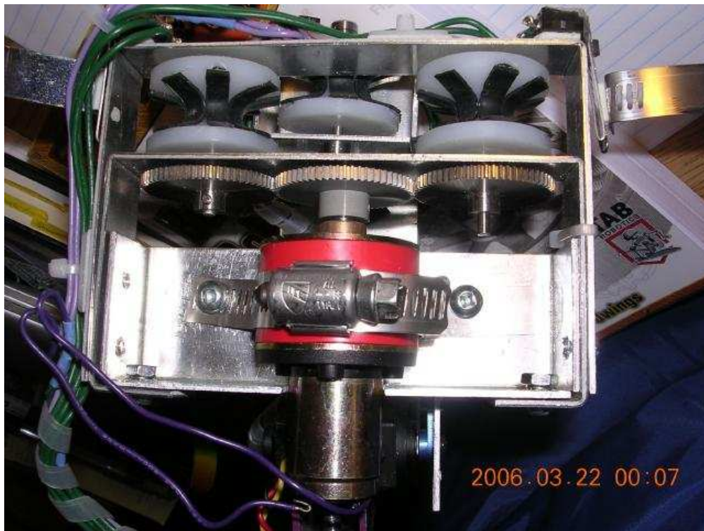
Figure 4: Lowered Chassis and Secured With Lock Washers and Nuts
