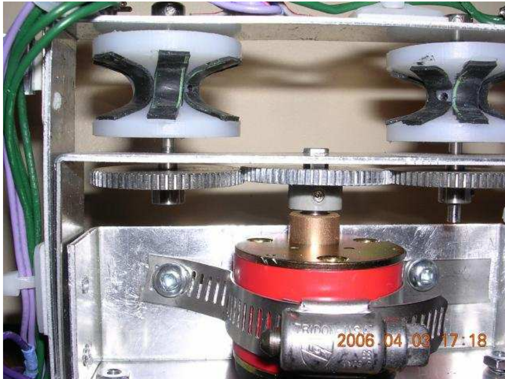
Figure 8: Follower Gear Working Loose
