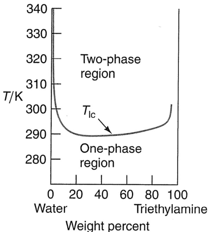
4. (a) From the phase diagram to the left (water-triethylamine), determine the ratio of the masses of the phases present at 295K, for a mixture containing 30.0 wt % triethylamine. (b) What are the respective compositions of the phases?
