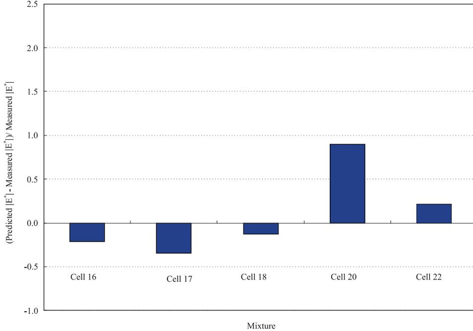
**Fig. 6.** Adjusting of the Witczak predicted  $|E^*|$  master curve using the  $|E_{40}^*|$ -GR model.
