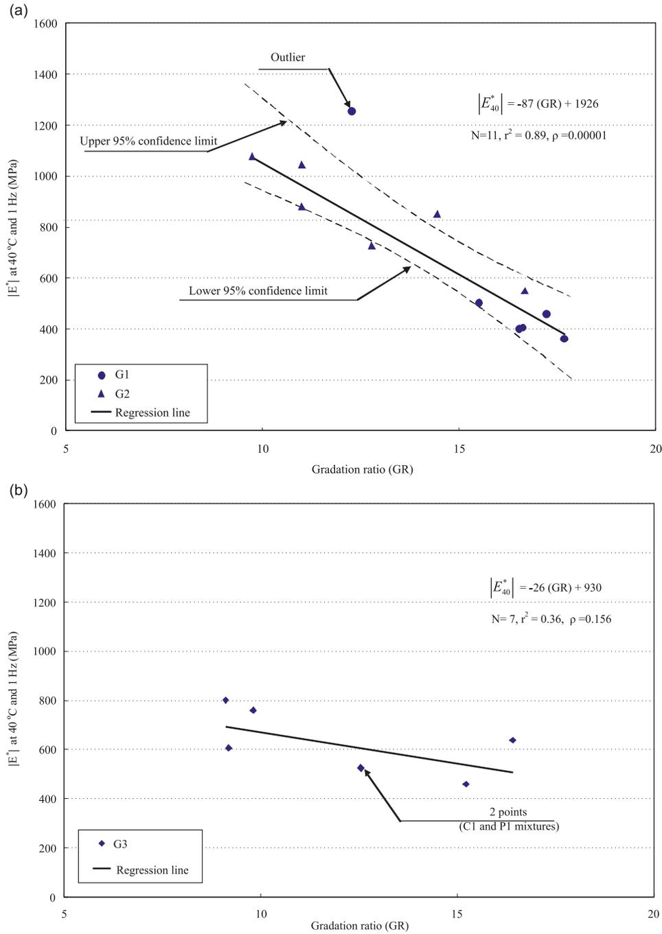
The statistics of the model confirm a significant relationship between  $|E_{40}^*|$  and GR for fine-graded mixtures. The data consists of 11 fine-graded mixtures with different aggregate gradations, aggregate sources, and binder grades. The material passing both the 0.075 mm and the 4.75 mm sieves are in the range of 3.5%–6.3% and 61.3%–77.5%, respectively. The model is simple since it includes one independent variable (GR) and it is rational since dynamic modulus decreases as GR increases.
