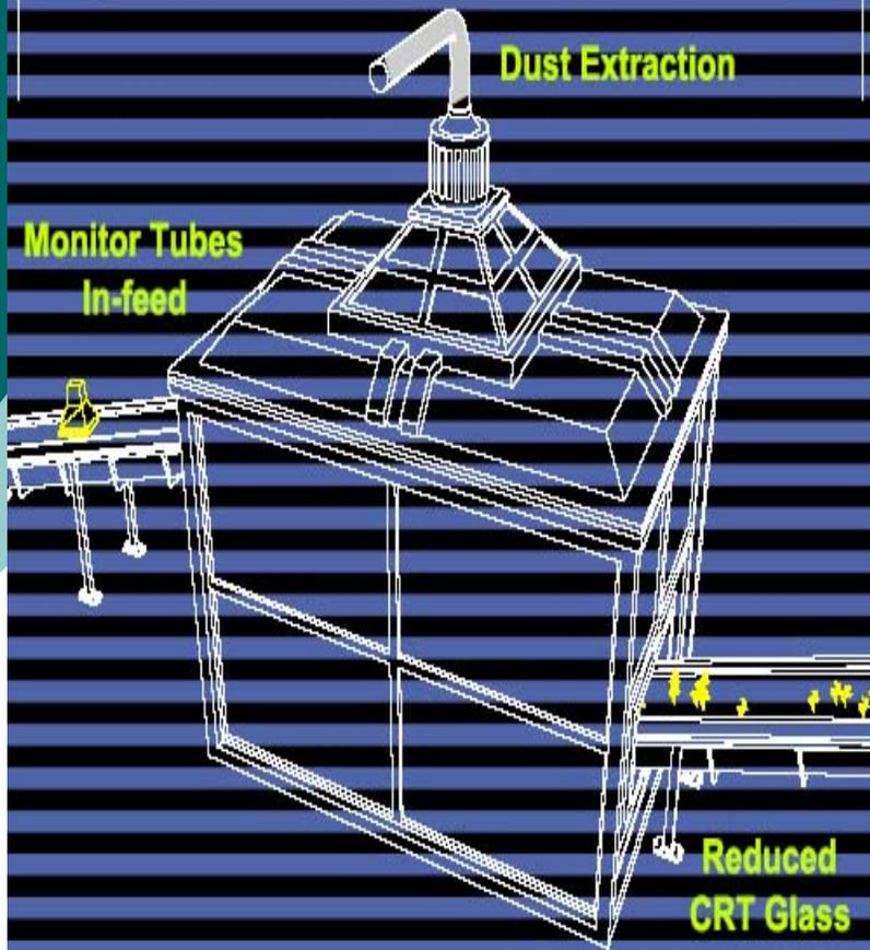
The first stage involves a controlled size reduction process. This process reduces the complete tube and screen down into smaller pieces.
