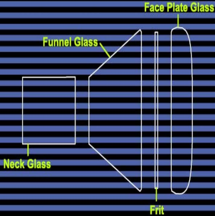
To achieve the maximum of recyclate, it is necessary to separate the "leaded" from "unleaded" glass i.e. the Face Plate from the Frit, Funnel and Neck.
