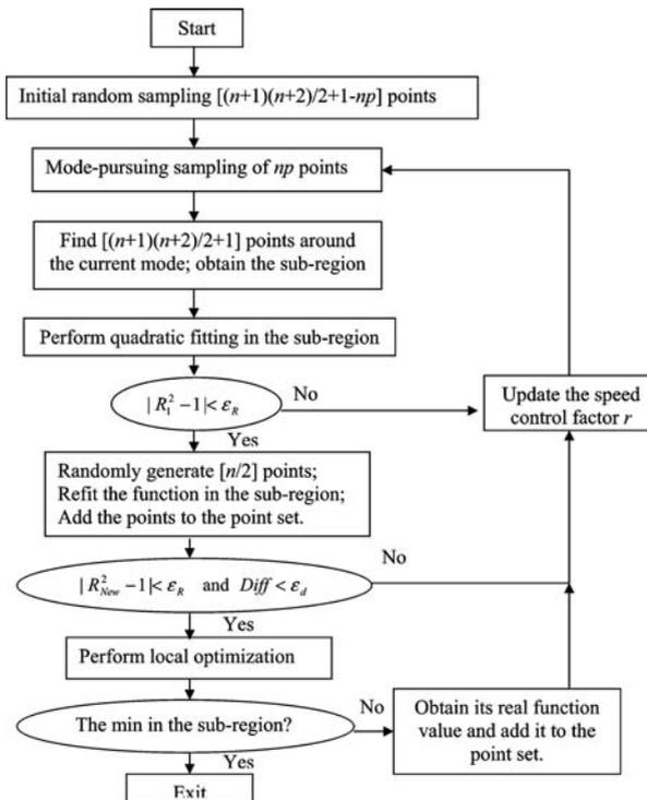
FIGURE 4 Flowchart of the proposed global optimization method.
