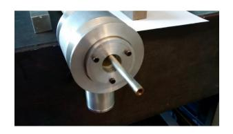
Insert the source rod into sample rod, carefully go through the glue joint of the G10 tube (the long sample tube was made by gluing two sections of G10 tubes together)
