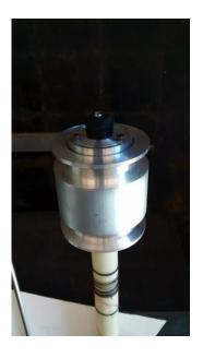
Twist the source rod onto the center screw of the rubber stopper to temporarily fix the source rod and prevent it accidently dropping into the sample rod when change samples
