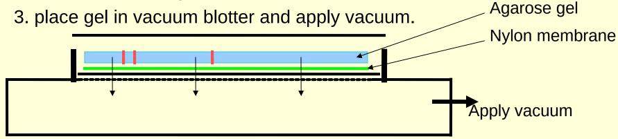
Buffer with soluble DNA pulled directly from gel onto membrane where DNA is bound replicating the separation pattern that was in the gel
