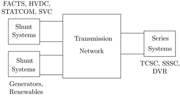
Figure 1. Representation of a power system
