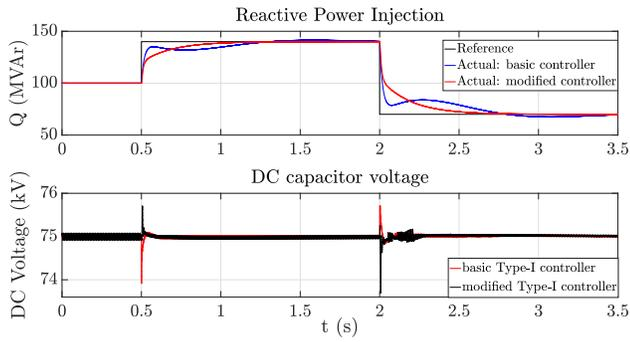
Figure 8. Step response of STATCOM Type-I controller ( $Q = 100$  MVar)
