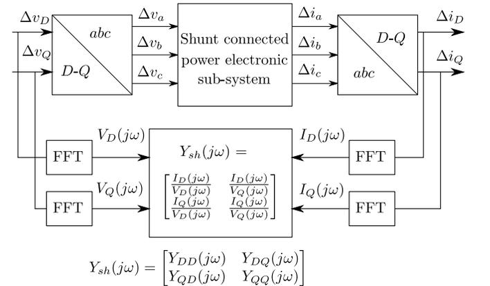
Figure 9. Frequency Scanning of shunt connected devices
