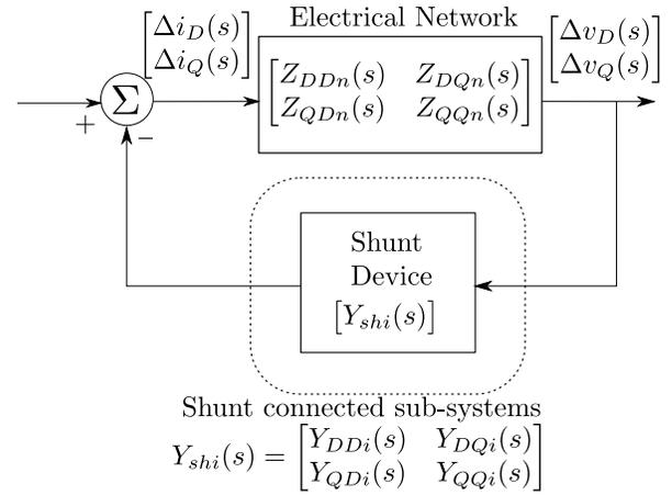
Figure 2. Schematic of feedback structure in power systems (shown here for only one shunt connected device)
