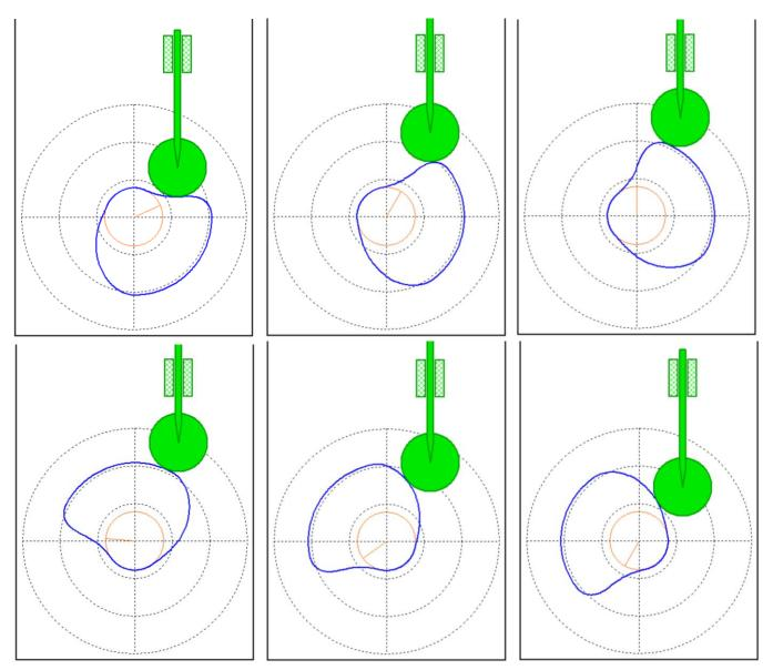
The pressure angle becomes quite large during the return motion as is evident in the last image; however, the return motion is often driven by an external force, say a return spring, and hence there is minimal risk of binding as a result of the large pressure angle.
