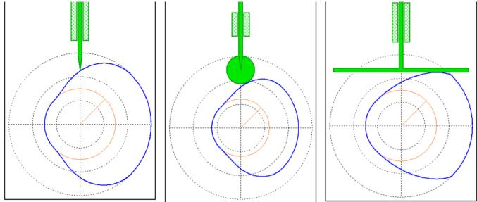
The issue with the third cam has been almost eliminated. Increasing the base circle makes the cam appear more round. Here is the cam for a knife edge follower with increasing base circle radius. All cases result in the same desired follower motion:
