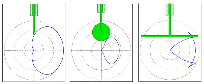
Remember that a knife edge can be thought of as a roller follower with a radius of zero and a flat plate follower as a roller follower with a radius of infinity.
