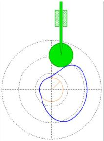
You can see that the cam profile changes ever so slightly and becomes asymmetrical with increasing offset distance. The pressure angle plots for case b) and c) are:
