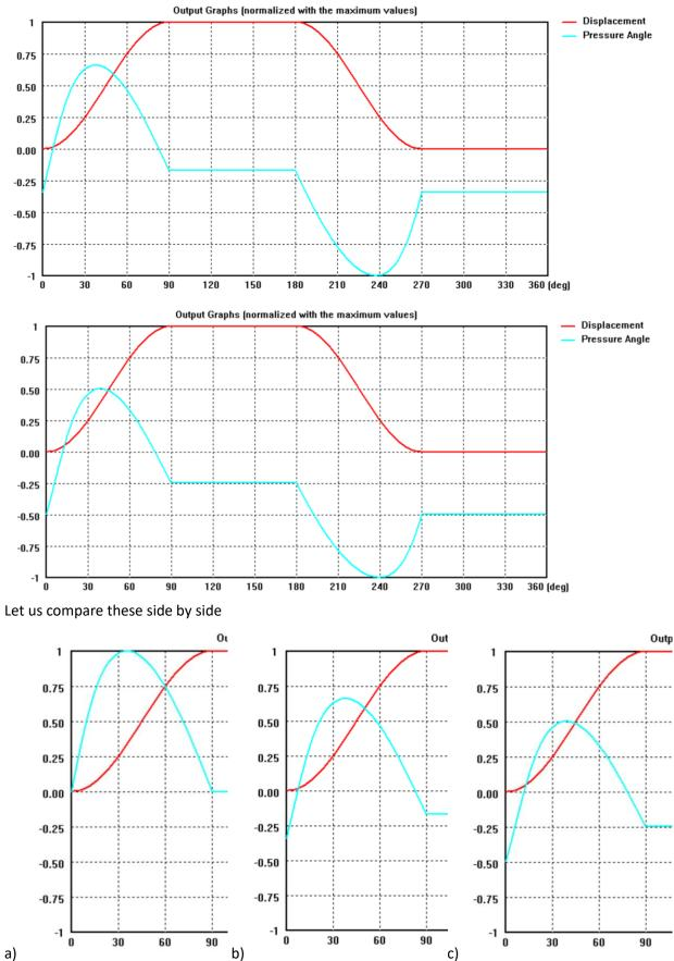
The decrease in the pressure angle during the rise is very clear. Here is a sequence of images when the offset distance is maxed out (equal to the roller follower radius plus the base circle radius):
