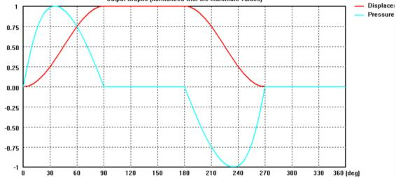
The pressure angle is the same during both the rise and the return. As I mentioned last time, the pressure angle can be manipulated through the use of an offset in the cam from the center position. This can be used to reduce the pressure angle during the rise motion and hence reduce the likelihood of binding of the cam. Here are three case: a) no offset b) some offset, and c) more offset:
