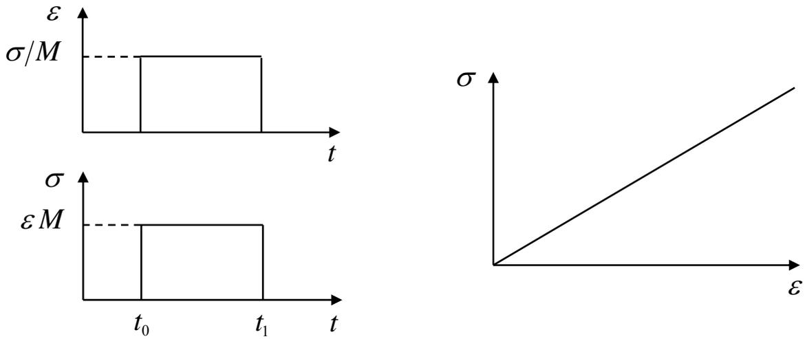
Fig. 2. Left: The strain-time diagram for a constant stress applied at time  $t_0$  and removed at time  $t_1$ . Right: The stress-strain diagram.
