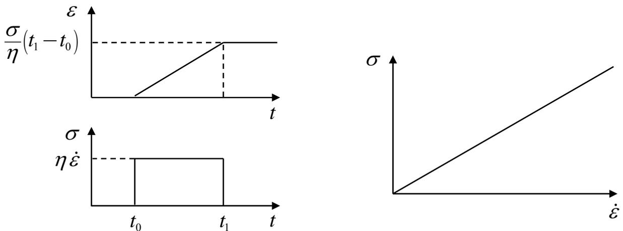
Fig. 4. Left: The strain-time diagram for a constant stress applied at time  $t_0$  and removed at time  $t_1$ . Right: The stress – strain-rate diagram.
