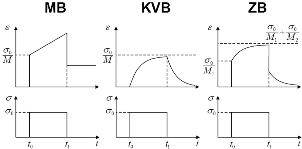
Fig. 6. Creep in Maxwell, Kelvin-Voigt and Zener (standard linear) bodies: strain-time diagrams for a constant stress applied at time  $t_0$  and removed at time  $t_1$ .
