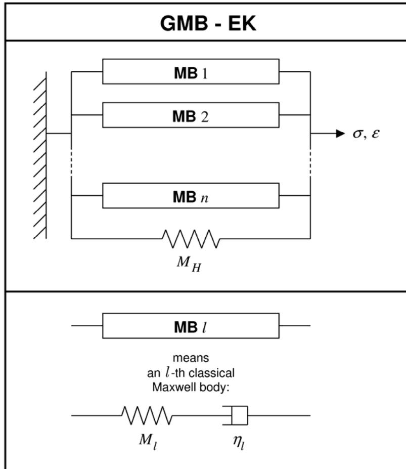
Figure 8. Rheological model of the Generalized Maxwell Body (GMB-EK) defined by Emmerich and Korn (1987).  $M_H$  and  $M_l$  denote elastic moduli,  $\eta_l$  viscosity.
