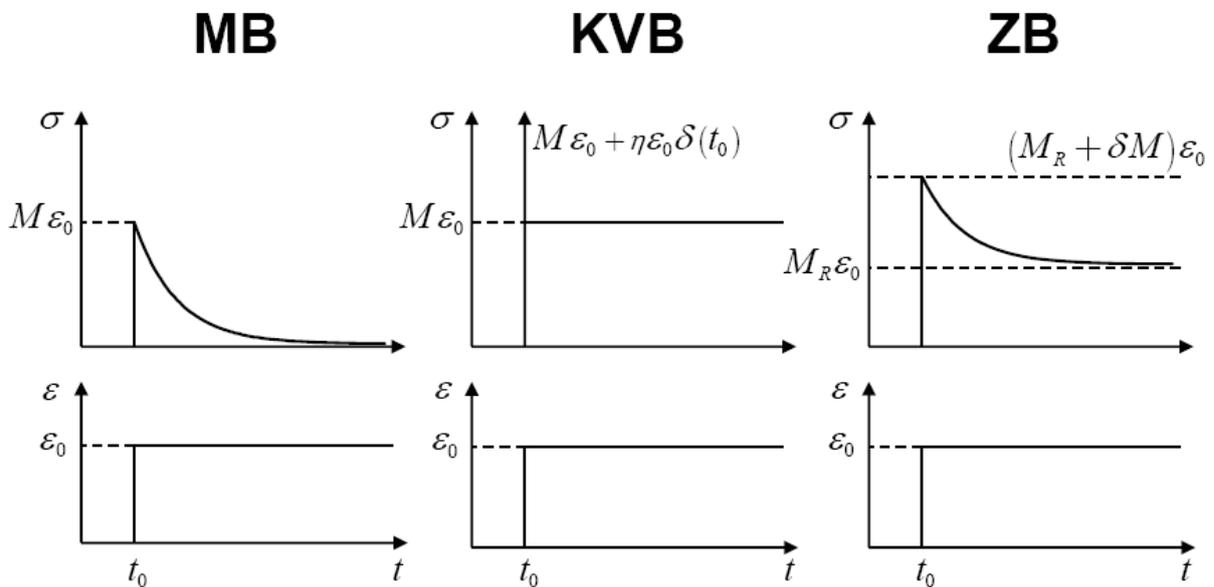
Fig. 7. Stress relaxation in Maxwell, Kelvin-Voigt and Zener (standard linear) bodies: stress-time diagrams for a constant strain applied at time  $t_0$ .
