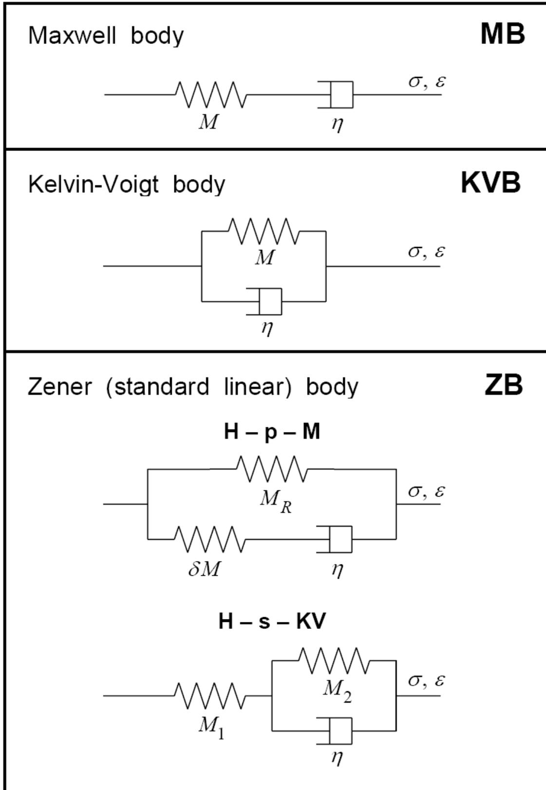
Fig. 5. The simplest rheological models of viscoelastic materials.
