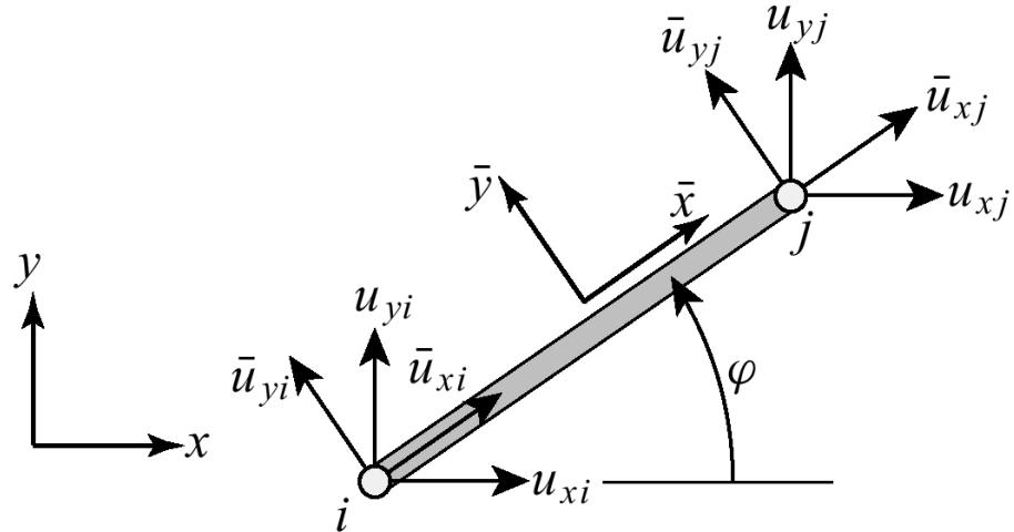
$$\begin{Bmatrix} \hat{d}_{x1} \\ \hat{d}_{y1} \\ \hat{\phi}_1 \\ \hat{d}_{x2} \\ \hat{d}_{y2} \\ \hat{\phi}_2 \end{Bmatrix} = \begin{bmatrix} c & s & 0 & 0 & 0 & 0 \\ -s & c & 0 & 0 & 0 & 0 \\ 0 & 0 & 1 & 0 & 0 & 0 \\ 0 & 0 & 0 & c & s & 0 \\ 0 & 0 & 0 & -s & c & 0 \\ 0 & 0 & 0 & 0 & 0 & 1 \end{bmatrix} \begin{Bmatrix} d_{x1} \\ d_{y1} \\ \phi_1 \\ d_{x2} \\ d_{y2} \\ \phi_2 \end{Bmatrix}$$
