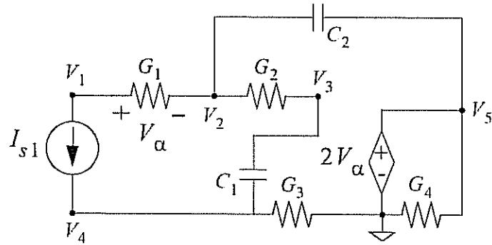
$$G_1 = 40S, G_2 = 20S, G_3 = 20S, G_4 = 10S, C_1 = 0.5F, C_2 = 0.6F, I_{s1} = 1A$$
