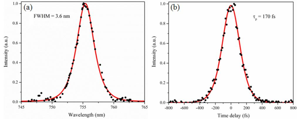
Fig. 3. Measured (a) spectrum and (b) autocorrelation trace of the pulses with fits assuming a  $\text{sech}^2$  profile.
