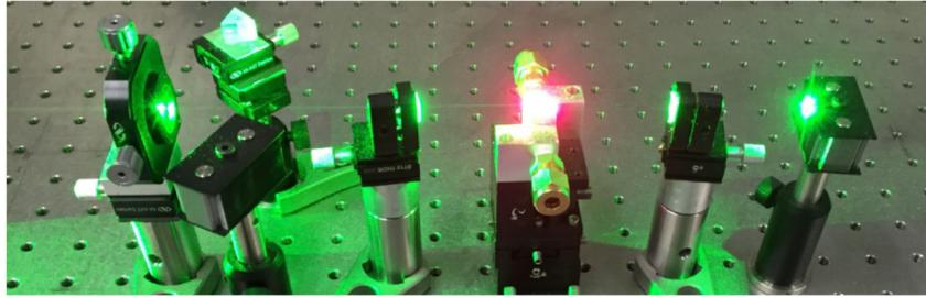
Fig. 5. Photograph of the pumped Alexandrite crystal in the laser cavity.
