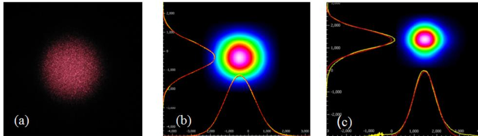
Fig. 4. Laser beam on paper surface (a) and its intensity profiles in the CW (b) and mode-locked (c) regimes. Beam size change in (b) and (c) is due to the different locations of the CCD camera in the CW and KLM experiments.
