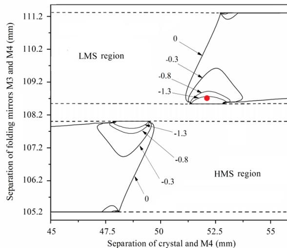
Fig. 2. Contour Magni plots for the used KLM resonator in the tangential plane. Red dot indicates the operating point. Dashed horizontal lines show stability edges. LMS - low misalignment sensitivity region, HMS - high misalignment sensitivity region of the resonator.
