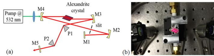
Fig. 1. (a) Schematic layout of the femtosecond KLM Alexandrite laser oscillator and a photograph of the laser crystal between the folding mirrors at low pump power. (b) The path of the pump light in the crystal near its center is clearly visualized by the excited fluorescence.
