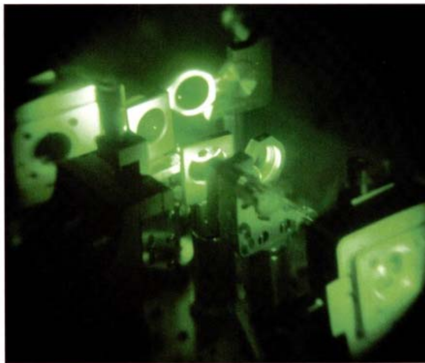
Researchers have designed an Yb:KGW laser. An infrared image of its laser head is shown.
