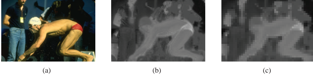
Figure 8: Example of normalized RGB probe function: (a) Original image [31], (b) normalized R over subimages of size 5 \times 5 , and (c) normalized R over subimages of size 10 \times 10 .
